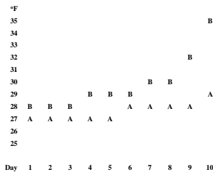
Figure 6.2. Trend chart of the temperature of shelled corn in two bins (A and B).
